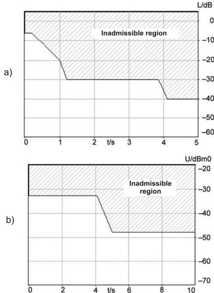
Fig. 8 — Time dependence of echo return loss  $L$  and echo signal level  $U$
