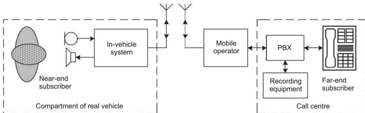
Fig. 5 — Test arrangement for subjective quality assessment of loudspeaker communication
