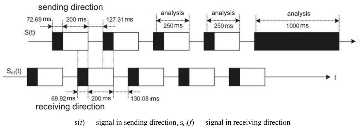
Fig. 12 — Test signal for evaluation of attenuation range in sending direction during double-talk
