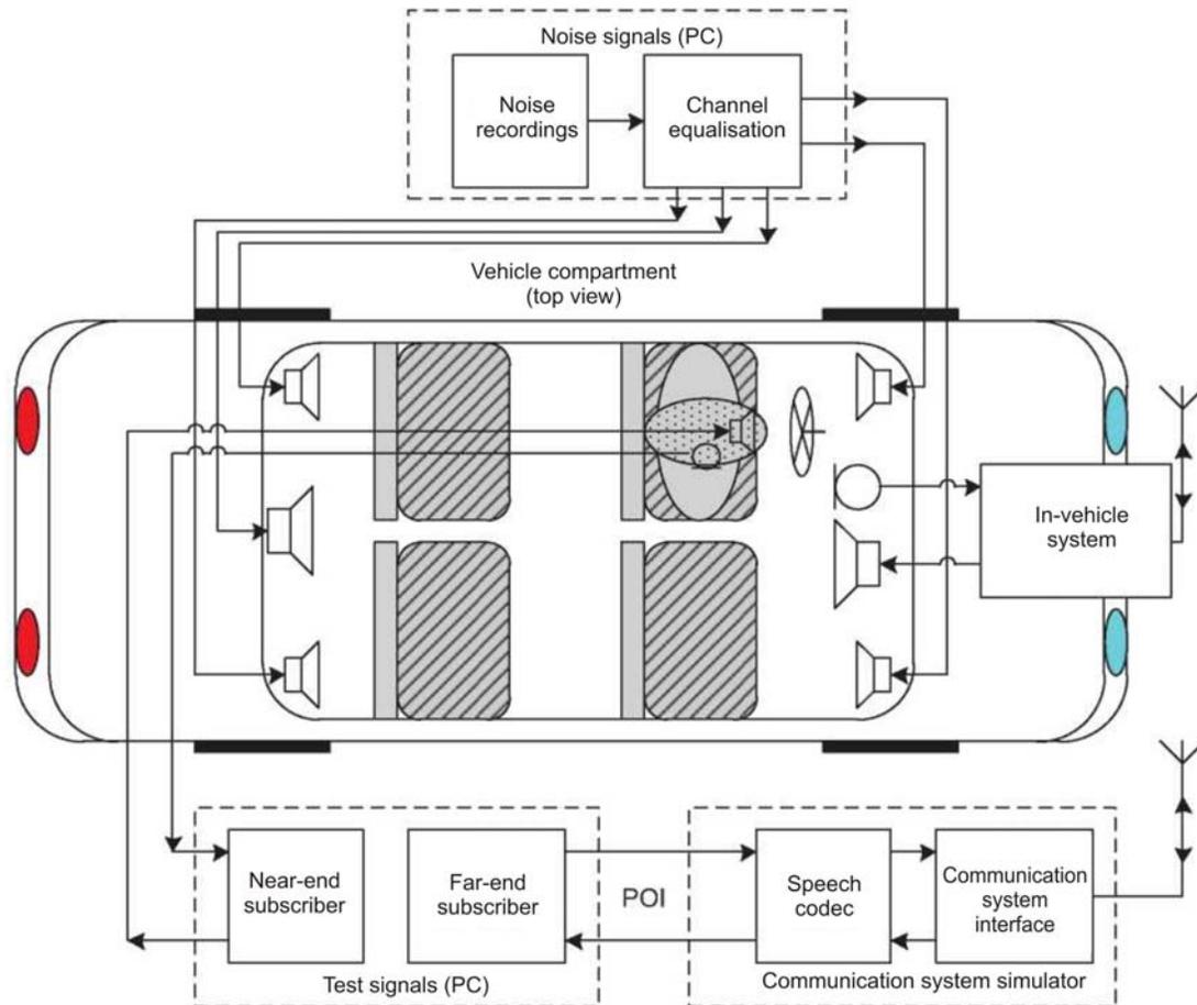
Fig. 3 — Testing equipment for simulation of external acoustic noise
