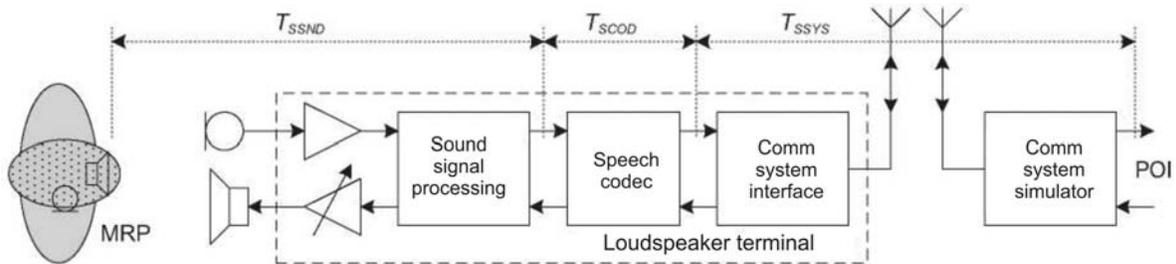
Fig. 6 — Signal propagation delay in sending direction
