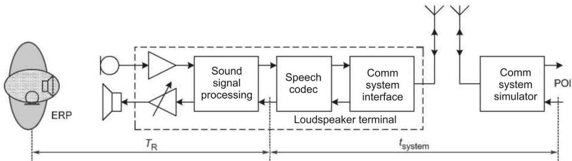
Figure 7 — Signal propagation delay in receiving direction
