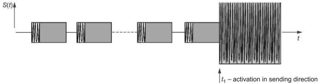
Fig. 11 — Waveform diagram of signals for measurement of attenuation in transmit channel [10].
