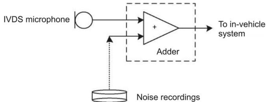
Fig. B.1 — Flow diagram of electric method used to inject previously recorded noises into test signals
