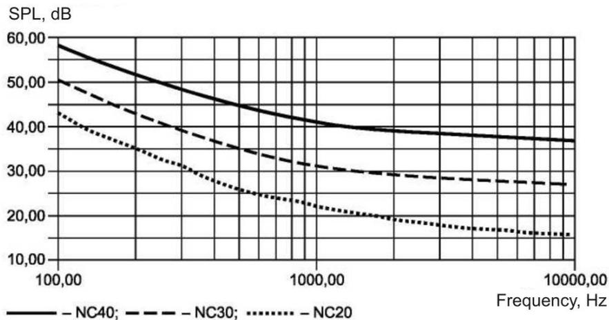
Figure 4 — Spectral density of ambient noise
