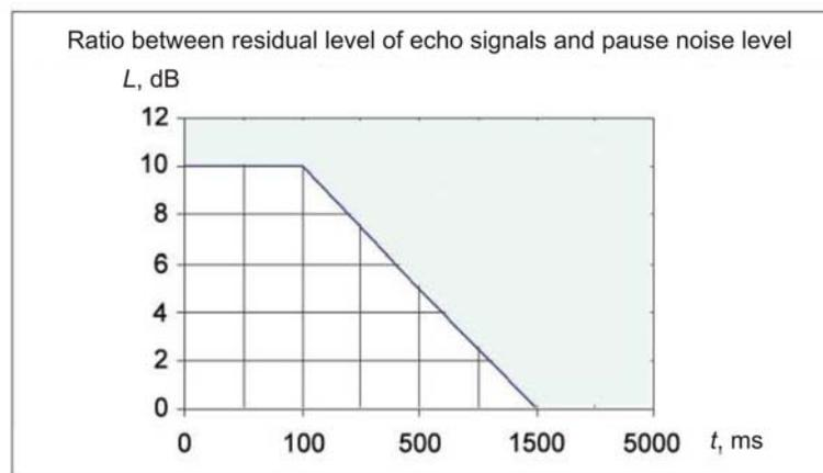
Fig. 9 — Time dependence of ratio between residual level of echo signals and pause noise level
