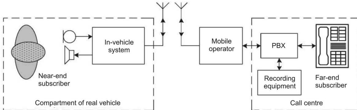
Figure 5 — Test arrangement for subjective quality assessment of loudspeaker communication
