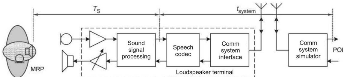
Figure 6 — Signal propagation delay in sending direction
