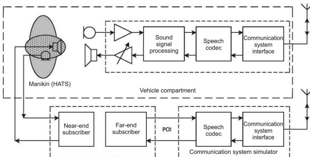
Figure 1 — Flow diagram of testing apparatus for tests of in-vehicle systems
