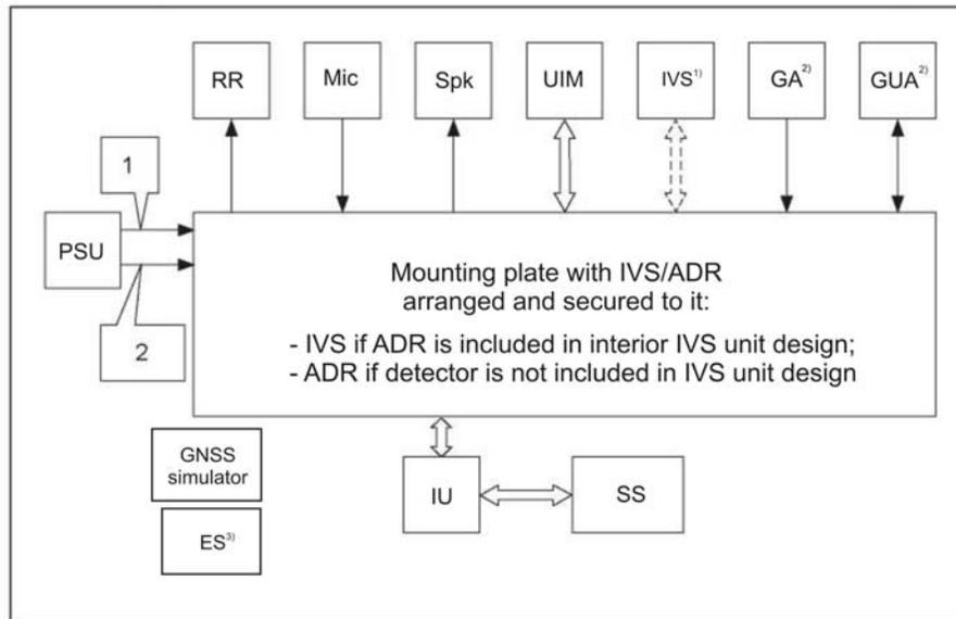
RR — radio recorder of vehicle; Mic — microphone; Spk — speaker; UIM — user interface module; ADR — automatic detector of RTA events; GA — GLONASS antenna; GUA — GSM/UMTS antenna; PSU — power supply unit (12/24 V); IU — interface unit; SS — simulator of road accident emergency response system; ES — emergency simulator; 1 — power cable; 2 — ignition circuit
