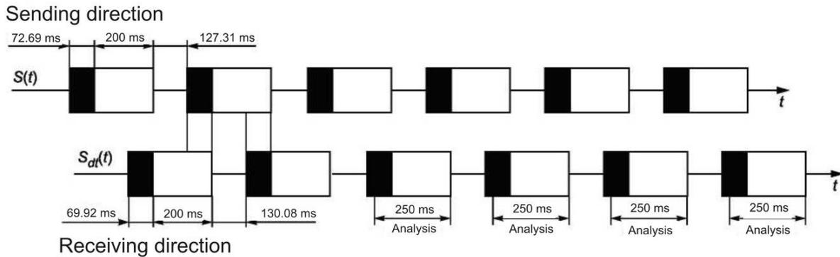
Figure 13 — Test signal for evaluation of attenuation range in receiving direction during double-talk
