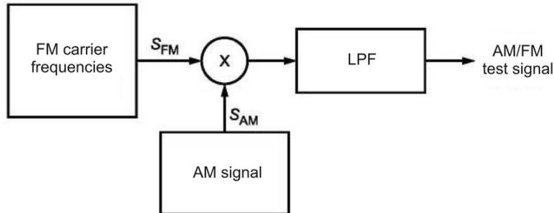
Figure 14 — Flow diagram of test signal generation based on AM/FM modulated sine sets
