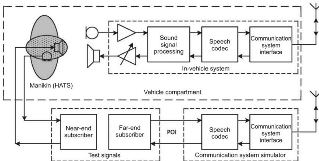
Fig. 1 — Flow diagram of testing apparatus for in-vehicle emergency call devices/systems
