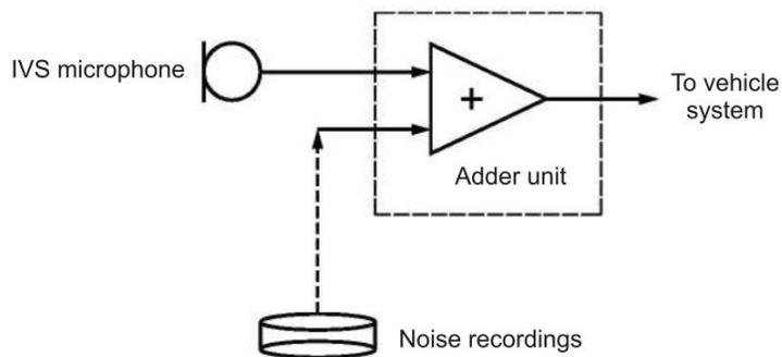
Figure B.1 — Flow diagram of electric method used to inject previously recorded noises into test signals
