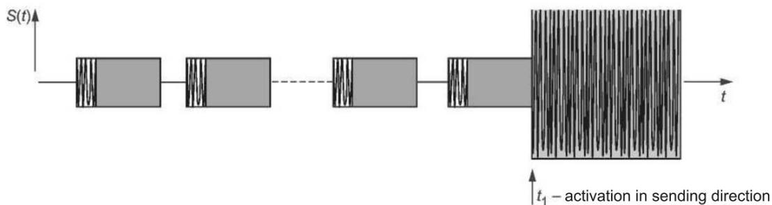
Figure 11 — Waveform diagram of signals for measurement of attenuation in transmit channel [31].
