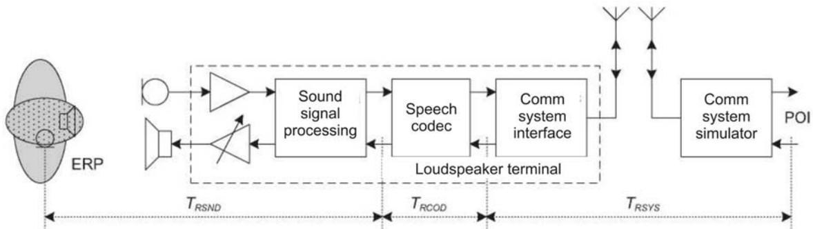
Fig. 7 — Signal propagation delay in receiving direction
