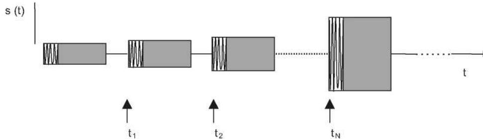
Fig. 10 — Test signal for evaluation of minimum activation level and channel activation time [10]
