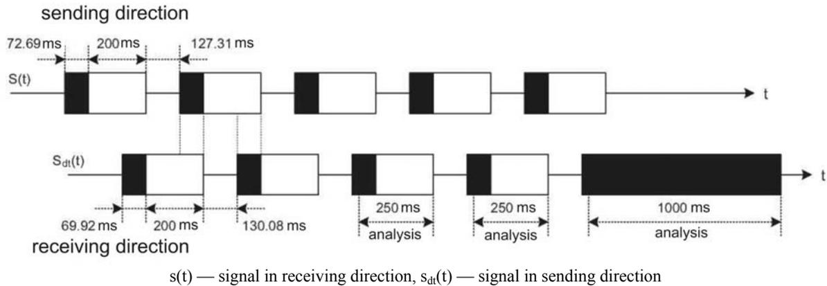
Fig. 13 — Test signals for evaluation of attenuation range in receiving direction during double-talk
