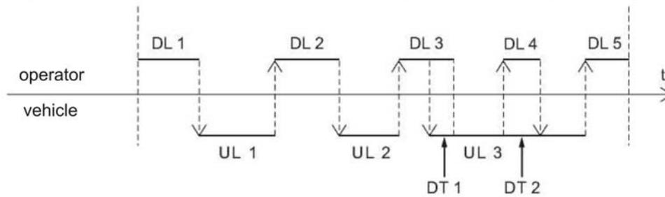
Fig. 15 — Playback sequence of recordings
