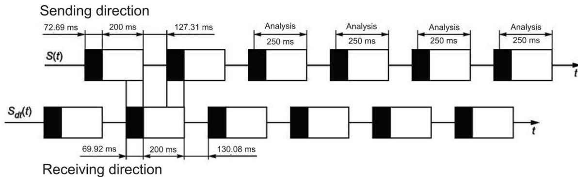
Figure 12 — Test signal for evaluation of attenuation range in sending direction during double-talk
