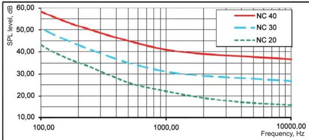
Fig. 4 — Spectral density of ambient noise
