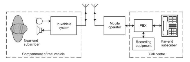
Figure 5 — Test arrangement for subjective quality assessment of loudspeaker communication
