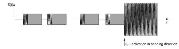
Figure 11 — Waveform diagram of signals for measurement of attenuation in transmit channel [31].
