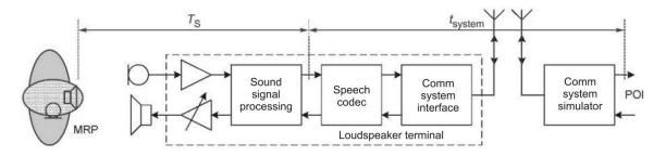
Figure 6 — Signal propagation delay in sending direction
