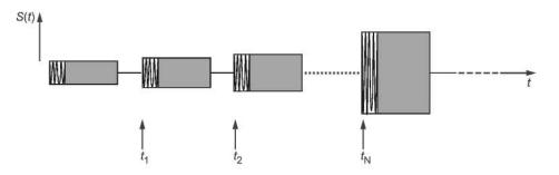
Figure 10 — Test signal for evaluation of minimum activation level and channel activation time [31]
