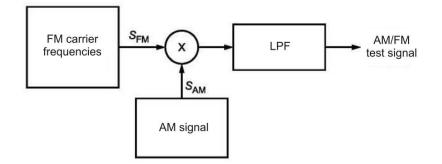
Figure 14 - Flow diagram of test signal generation based on AM/FM modulated sine sets
