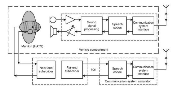
Figure 1 — Flow diagram of testing apparatus for tests of in-vehicle systems
