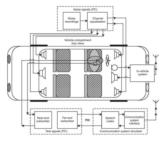
Figure 3 — Testing equipment for simulation of external acoustic noise
