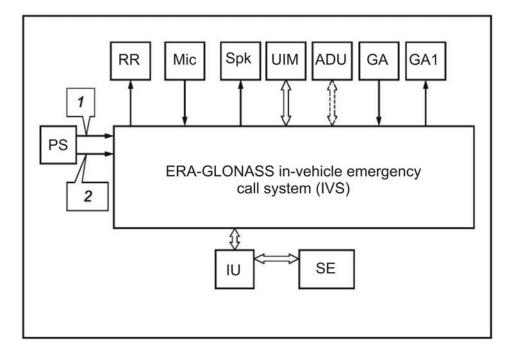
RR — radio recorder of vehicle; Mic — microphone; Spk — speaker; UIM — user interface module; ADU — accident detector unit; GA —GLONASS antenna; GA1 — GSM/UMTS antenna; PS — power supply (12/24 V); IU — interface unit; SE — ERA-GLONASS system emulator; *I* — power cable; *2* — ignition circuit
