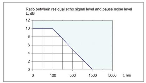
Figure H.2- Time dependence of ratio between residual echo signal level and pause noise level [3]
