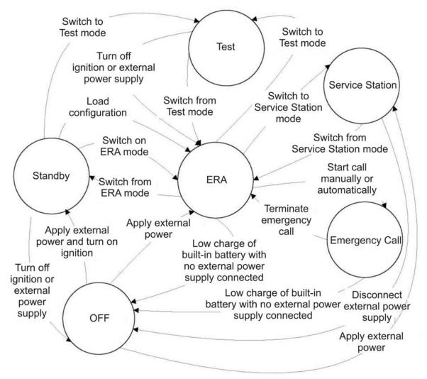
Figure 1 - State diagram of in-vehicle emergency call system in auxiliary equipment configuration
