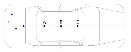
Figure E.1 - Recommended arrangement of detector of RTA events
