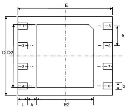
Figure 3 - MFF2 form-factor, bottom view
