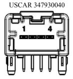
Figure G.1 - Recommended connector for coupling to RS 485 bus
