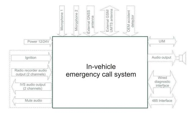
Figure D.1 – Example of IVS connection to on-board audio system
