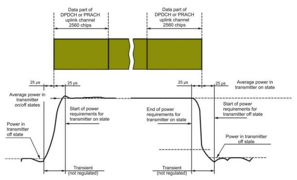
Figure B.1 — Transmitter emission on/off temporal pattern for UMTS 900 modem for physical random access channel
