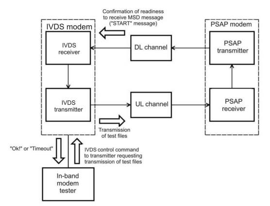
Figure F.7 — General test arrangement for check of HLACK message reception
