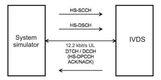
Figure E.2 — Arrangement for IVDS-UMTS tests pertaining to evaluation of maximum output power in HSDPA mode
