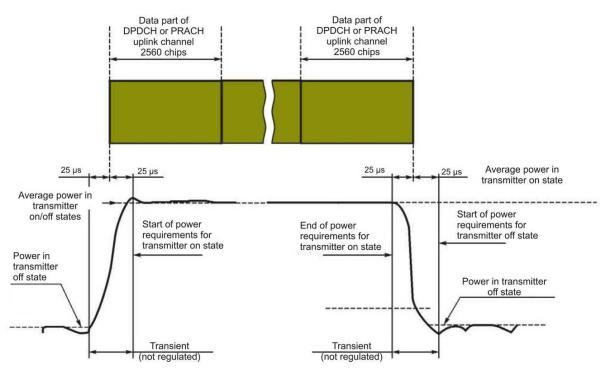
Figure B.2 — Transmitter emission on/off temporal pattern for UMTS 900 modem for other channels
