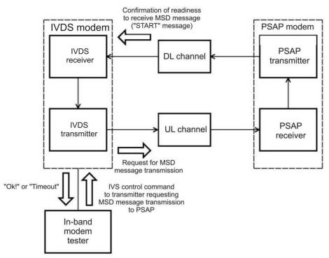
Figure F.6 — General test arrangement for check of PUSH message transmission/reception from/to in-band IVDS modem
