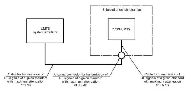
Figure E.1 — Arrangement for IVDS-UMTS tests using UMTS system simulator
