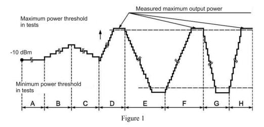
8) From the system simulator, send a sequence of 50 TPC commands consisting of "1". Each fifth command must be "TPC cmd+1" with a step size of 1 dB, and the remaining ones must be "TPC cmd 0".
