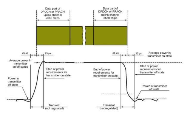
Figure 4 — Transmitter emission on/off time pattern for all other channels
