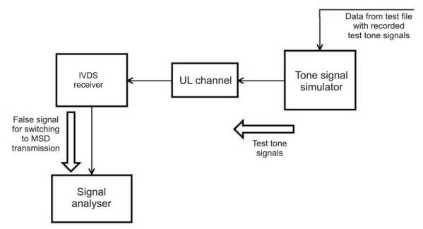
Figure F.5 — General test arrangement for check of false emergency call detection with signalling tones present on receiver input of in-band modem
