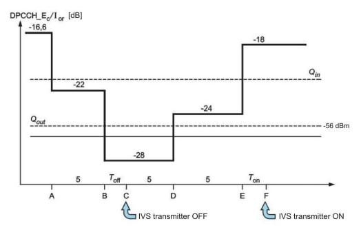
$Q_{out}$  is the low threshold of the received signal quality. If the quality index of the received signal falls below  $Q_{out}$ , the IVDS-UMTS transmitter will turn off.
