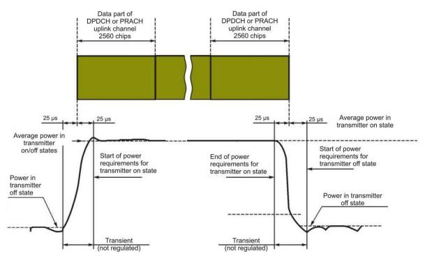
Figure C.1 — Transmitter emission on/off temporal pattern for physical random access channel
