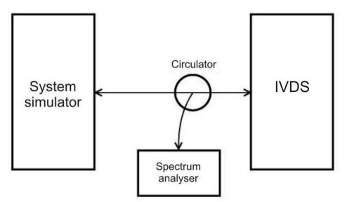
Figure E.3 — Arrangement for IVDS-UMTS tests pertaining to evaluation of maximum permitted levels of IVDS-UMTS out-of-band emissions
