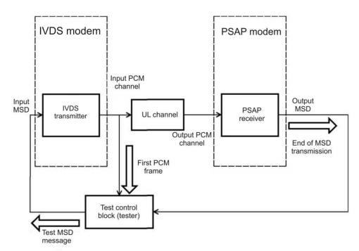
Figure F.2 — General test arrangement for evaluation of average MSD transfer time for various AMR and GSM-FR speech codecs
