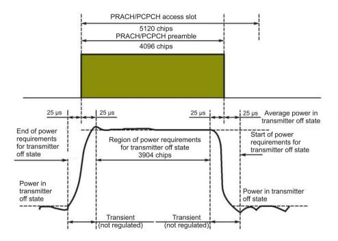
Figure 3 — Transmitter emission on/off time pattern for physical random access channel
