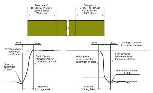
Figure C.2 — Transmitter emission on/off temporal pattern for other channels
