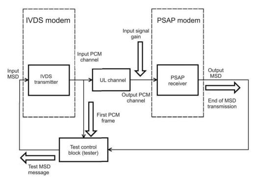
Figure F.4 — General test arrangement for measurement of MSD transmission time for different values of PCM signal gain
