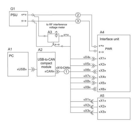
A1 — PC; A2 — USB-to-CAN module; A3 — V-shaped dummy on-board network (see Table 2); A4 — interface unit; A5 — IVDS under test; G1 — power supply unit; L1 — 5A air-core inductance coil; P1 — oscilloscope; *I* — cable; 2, 3 — ML-4G wire
