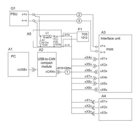
A1 — PC; A2 — USB-to-CAN module; A3 — interface unit; A4 — IVDS under test; A5 — dummy on-board network; G1 — power supply unit; L1 — 5A air-core inductance coil; P1 — oscilloscope; 1 — cable; 2, 3 — ML-4G wire
