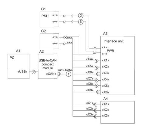
A1 — PC; A2 — USB-to-CAN module; A3 — interface unit; A4 — IVDS under test; G1 — power supply; G2 — test generator of impulse interference in vehicle on-board network; *I* — cable; 2, 3 — ML-4G wire
