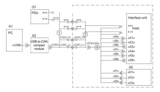
A1 — PC; A2 — USB-to-CAN module; A3 — interface unit; A5 — IVDS under test; G1 — power supply unit; 1 — CAN-OUT cable; 2 — CAN-IN cable, 3 — cable
