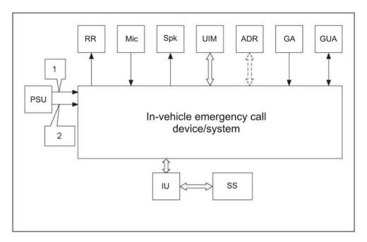
RR — radio recorder of vehicle; Mic — microphone; Spk — speaker; UIM — user interface module; ADR — automatic detector of RTA events; GA —GLONASS antenna; GUA — GSM/UMTS antenna; PSU — power supply unit (12/24 V); IU — interface unit; SS — simulator of road accident emergency response system; *I* — power cable; *2* — ignition circuit
