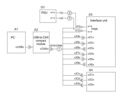
A1 — PC; A2 — USB-to-CAN module; A3 — interface unit; A4 — IVDS under test; G1 — power supply; *1* — cable; 2, 3 — ML-4G wire
